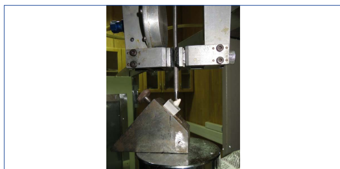
[Table/Fig-1]: Mounted specimen at an angle of 130°.
